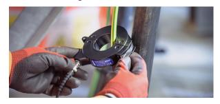
**The CableData Monitor**® allows us to continuously monitor and report to you on PD activity in live cable networks. This helps to reduce the need for disruptive maintenance shutdowns by highlighting high risk areas in ample time for repairs and replacements to be made if necessary. The system is a fully integrated modular system with up to 20 nodes and each system is capable of monitoring up to 180 cables.
